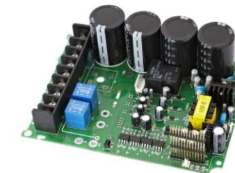
Inverter Drive Board
